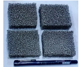
ARCI produced 10 PPI reticulated SiC foams
